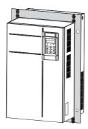
b. Fasten the AC drive onto the backplate of the control cabinet from the front of the control cabinet.
