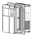
b. Fasten the AC drive with the bracket mounted onto the mounting backplate of the control cabinet.
