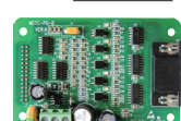
MCTC-PG-D Quadrature incremental encoder card 5 Vdc supply, female 15-way D-type connector (A, A l , B, B l , 0 V @ 5 V HTL)
