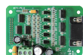
MCTC-PG-D Quadrature incremental encoder card (A, A l , B, B l ) with UVW commutation signals 5 Vdc supply, female 15-way D-type connector
